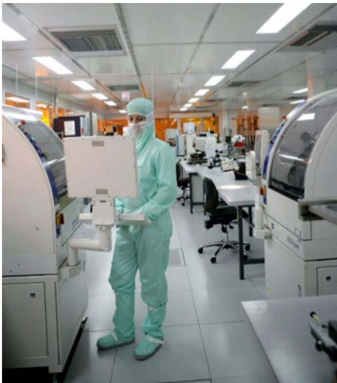
The ISO Class 7 clean room in Valtronic's Swiss facility includes flow boxes where workers can reduce contamination to ISO Class 5 levels as needed.
