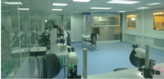
Valtronic Morocco operates both ISO Class 7 microbial-controlled and Class 8 clean rooms.
