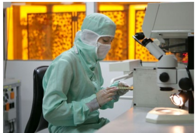
The ISO Class 7 clean room in Valtronic's Swiss facility includes flow boxes where workers can reduce contamination to ISO Class 5 levels as needed.
